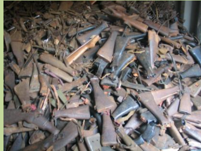
A picture of pieces of firearms after destruction using the Macyntire MC 4000 Shears machine
